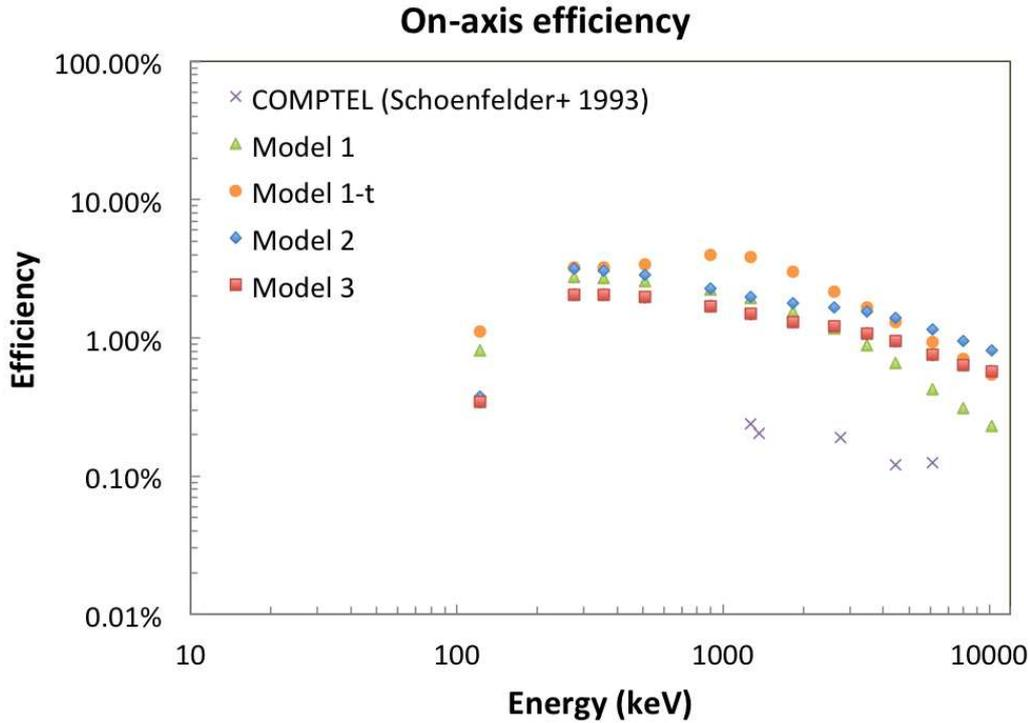
**Fig. 2.** The on-axis efficiency of the four instrument models. The COMPTEL efficiency (Schoenfelder et al. 1993) is plotted for comparison. We note that the COMPTEL ones are with photo-peak energy cut, while ours are without. Typically energy cut yields a reduction of a factor of 2 or 3.
