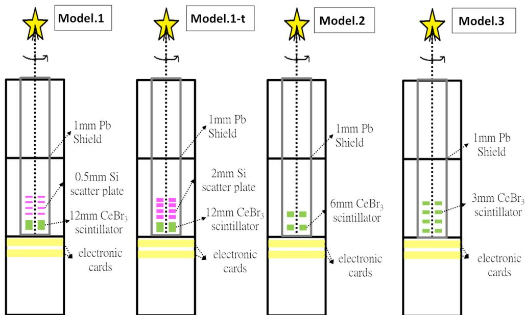
**Fig. 1.** The four instrument models studied in this paper. The numbers shown in this figure are all for thickness. See the main text for more descriptions. The instrument with its shield is located in the upper 2 U of a 3-U cubesat. When pointed towards Cyg X-1 for observation, a slow rotation around the pointing direction is desired for eliminating systematic bias for the azimuthal scattering angle distribution, which is of essential importance in polarization measurement.
